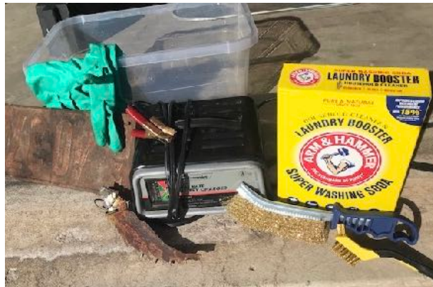
Above: Assembled materials for electrolysis, Clockwise from top. Plastic tub, rubber gloves, washing soda, wire brushes, battery charger, sacrificial steel on a hook. Photo provided by Don Neidigk, February, 2024.
