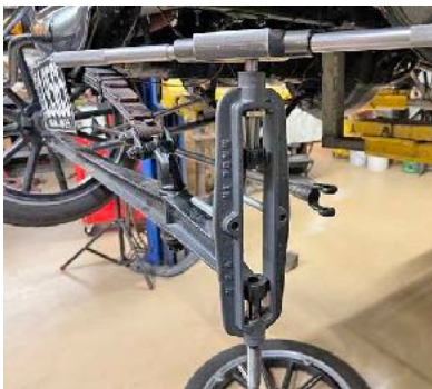
Stevens Axle Bushing Fixture in place on Mark Dominguez's Tudor sedan. Photo by Mark Wing, January, 2024.
