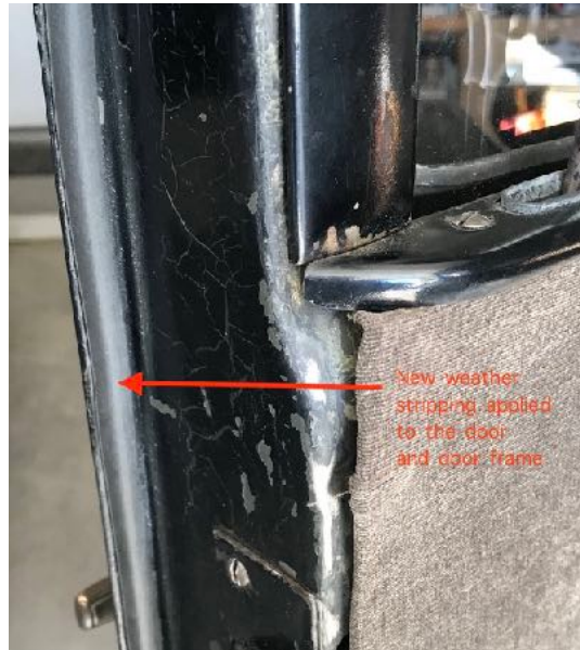
Photo Above: M-D self-adhesive rubber weather stripping installed around the '27 Coupe door and door frame on the body. Note of Caution: Exhaust fumes could build up in the cab with the windows and doors tightly sealed, so Don thinks he might have to install a "real tail pipe, not just a deflector." Photo provided by Don Neidigk, taken December, 2023.
