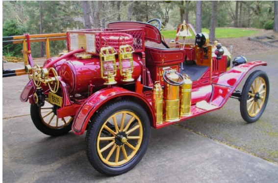
Rear View showing the chemical tanks and hose for the Wes Melo '15 Model T chemical car. Photo from Reference 4. below, screen grab by Marilyn Duncan.
