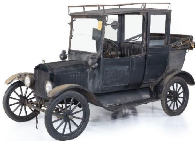
Ford Model T taxicab with a landaulet style body with a fixed roof for the driver and a convertible roof for the passengers. Photo screen grab from the Henry Ford Taxicab digital collection, 2023.
