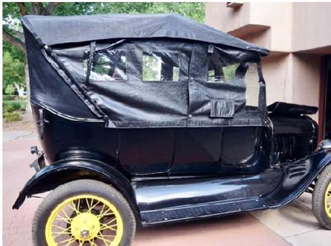
Dave Ferro's 1924 Touring car after top/rear curtain repair and installation of remodeled-side curtain panels. Photo by Paul Duncan May, 2023.
