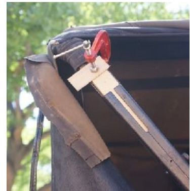
Above: Detail of rear bow wood tack strip repair. Below: Dave Ferro trimming and reinforcing the top pad and refitting the back curtain after adding an extension to the material. Photos by Paul Duncan, May, 2023.
