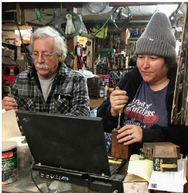
Larry Azevedo with the EECT 3 in 1 coil adjusting tool and Jessica Lance using the software information to adjust her sedan coil points. Photo by Paul Duncan, November, 2022.
