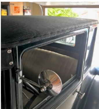
Picture 7: New vinyl top, trim and newly-replaced window glass.
