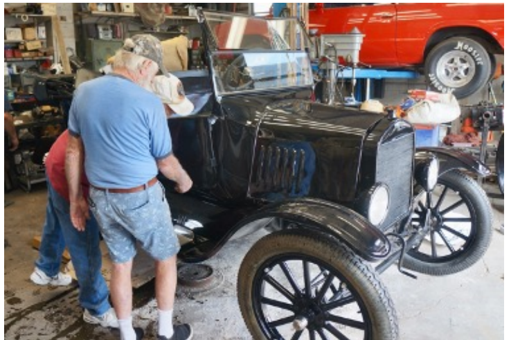
Above: Jim Glover inspects his T for damage after being pulled back upright by the come along winch. The windshield frame bent and the glass broke. Photo by Paul Duncan, September, 2022.
