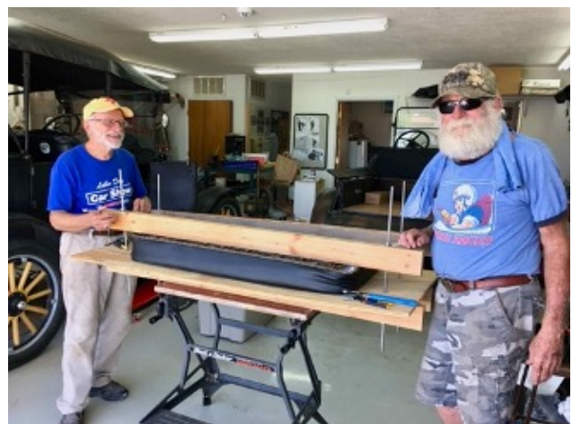
Paul Duncan (L) and Jim Glover (R) using the seat cushion compression table to install upholstery. Photo by Marilyn Duncan, July, 2022
