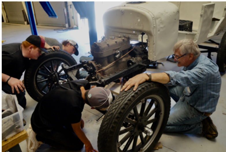
Right: Dave Ferro and Valencia High School students working to mount the front wheels on their Model T Touring project car. Photo by Paul Duncan, May 2022.
