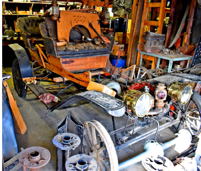
1909 Model T in parts was recently purchased by Mark Wing. Photo shows the T in the California garage prior to loading into the trailer. The early engine block is in front of the car (barely visible). The early "no rivet" clamshell rear differential is the primed unit sitting between the front wheels. The transmission is laying on the frame in the radiator location. Photo by Mark Wing.
