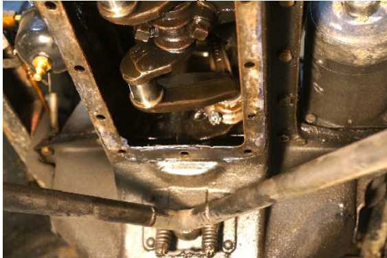
The #4 piston is located back beyond the opening of the inspection plate and difficult to reach.
