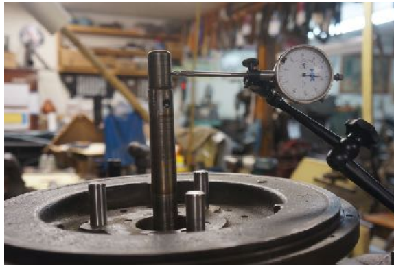
Checking the concentricity of the transmission shaft with a dial indicator gauge. Photo by Paul Duncan
