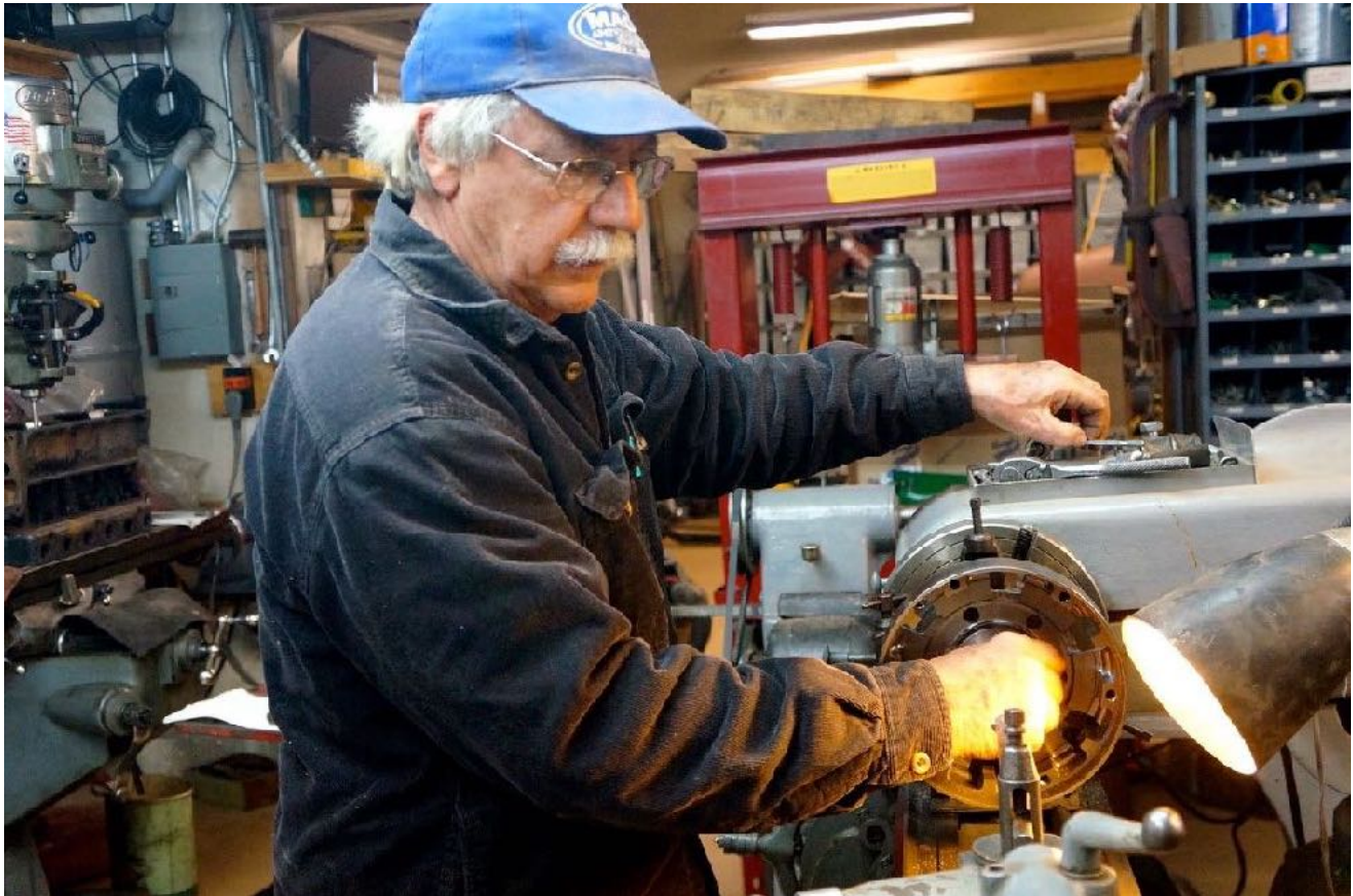
Larry Azevedo working on a lathe in his Shop. He is making final adjustments on the brake drum bushing during rebuild of the Duncan 1926/1927 engine. See Cover Story Page 3. Photo by Paul Duncan, December, 2020
