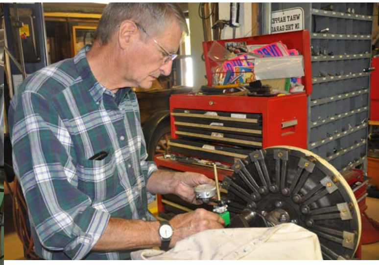
Dave aligning magneto magnets vvv
