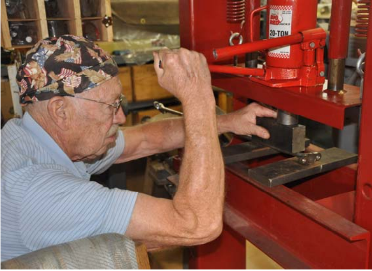
^^^ Neil straightening a steering arm
